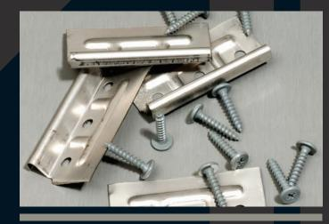
The clips are fixed to the substrate using two Met-Seam® grade 302 HQ stainless steel screws per clip. The clips are then concealed by the next consecutive panel thus hiding all fixings.
