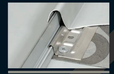
The Seam over cloak fits over the Locking Leg and snaps into place. The Locking Leg is profiled with an anti-siphon design which doubles up to eliminate capillary action in the joints and forms the 'Receiver' to which the MS secret fixing clip is placed to secure the panel to the substrate.
